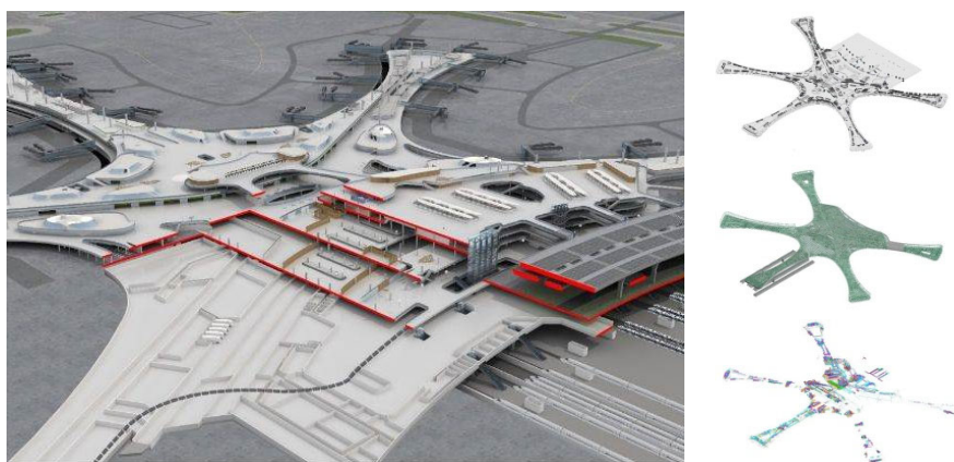
Figure 1. Application of BIM Technology in Daxing Airport (Revit full discipline design model)
