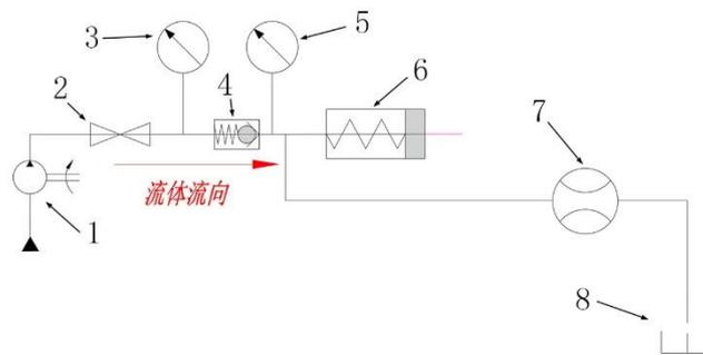
1- Hydraulic pump; 2- Manual valve; 3, 5- Pressure gauge; 4- Check valve; 6- Miniature cylinder; 7- Flowmeter; 8- tank
