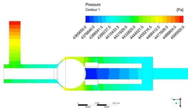
(a) Initial pressure contours at thrust 50N
