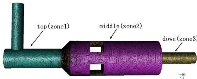
Fig 3. Grid model of check valve
