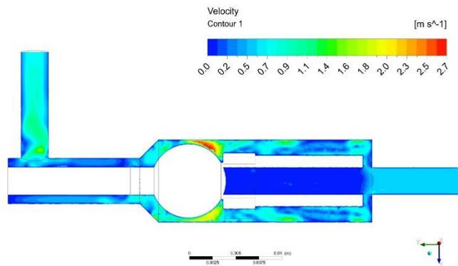
(b) Velocity contours after stabilization at thrust 50N
