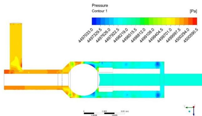
(b) Pressure contours after stabilization at thrust 50N
