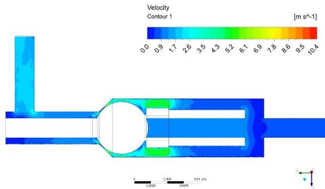
(a) Initial velocity contours at thrust 50N
