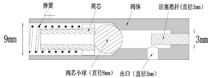
**Fig 1.** Schematic diagram of check valve structure
