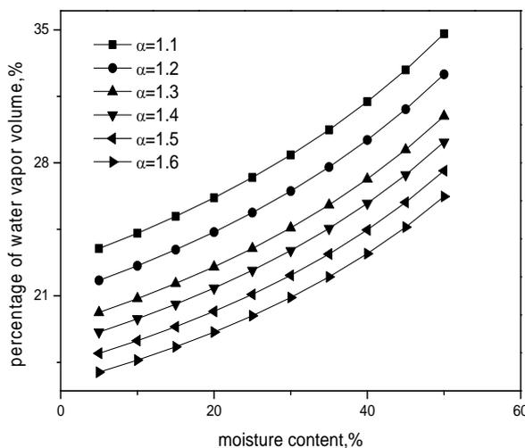
**Fig 2.** Relationship between moisture content of enteromorpha clathrata, excess air coefficient and volume fraction of water vapor
