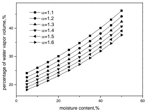
**Fig 3.** Relationship between moisture content of rice straw, excess air coefficient and volume fraction of water vapor
