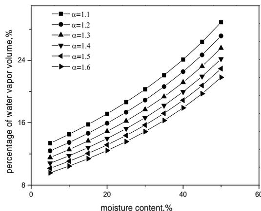
**Fig 1.** Relationship between moisture content of pine wood, excess air coefficient and volume fraction of water vapor
