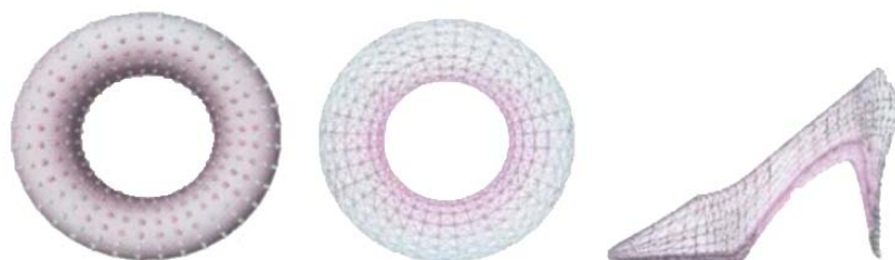
(a) Convex and concave vertex (b) Convex and concave facet (c) Saddle facet
