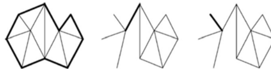
(a)BoundaryEdge deletion (b)The edge that cannot be deleted (c)The edge that can be deleted
